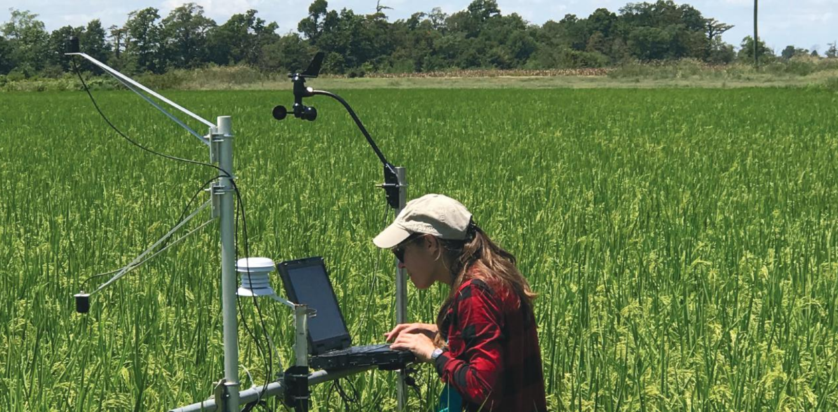
Image caption: Post-doctoral research associate, Beatriz Moreno Garcia, works with the Eddy Covariance equipment in a rice field in the Arkansas Delta. Garcia works for Dr. Benjamin Runkle, University of Arkansas professor of Biological and Agricultural Engineering.
